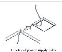
· Minimise the length of power cable run between the unit and the power source. Secure cable to prevent vibration damage.
