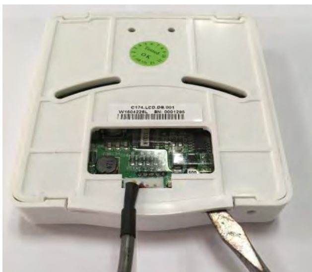
Figure 7-Pop off the rear cover of the interface using a flat head screwdriver or similar
