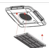
Install the air filter as shown:
