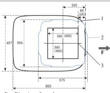
• The figure below shows the footprint of BELAIRE air-conditioner and the clearance required on the ceiling for the plenum installation. Measure from the reference position of the 360×360mm (400×400mm) square hole.Remember to add 100mm clearance around roof top unit perimeter.
