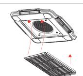
Install the air filter as shown: · Insert the two large tabs on the filter in the
