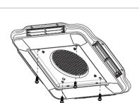
• Fix the plenum assembly on the plenum mounting bracket with four ST4×19 pan
