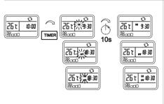
• Press the "TIMER" key repeatedly until either the ON or OFF or both symbols are flashing depending on which timer mode is preferred. To confirm the selection wait 10 seconds until the symbol stops flashing and lights up permanently-The clock time shows
